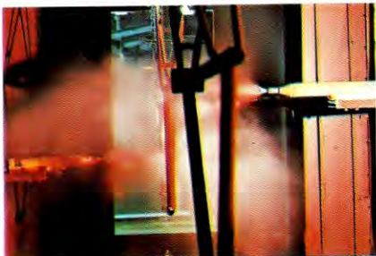
View inside automatic booth showing opposing electrostatic guns applying powder.
