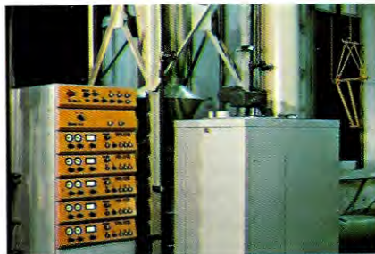
Powder feed rate and voltage for each gun are individually controlled from separate drawer-mounted control panels in central rack.
