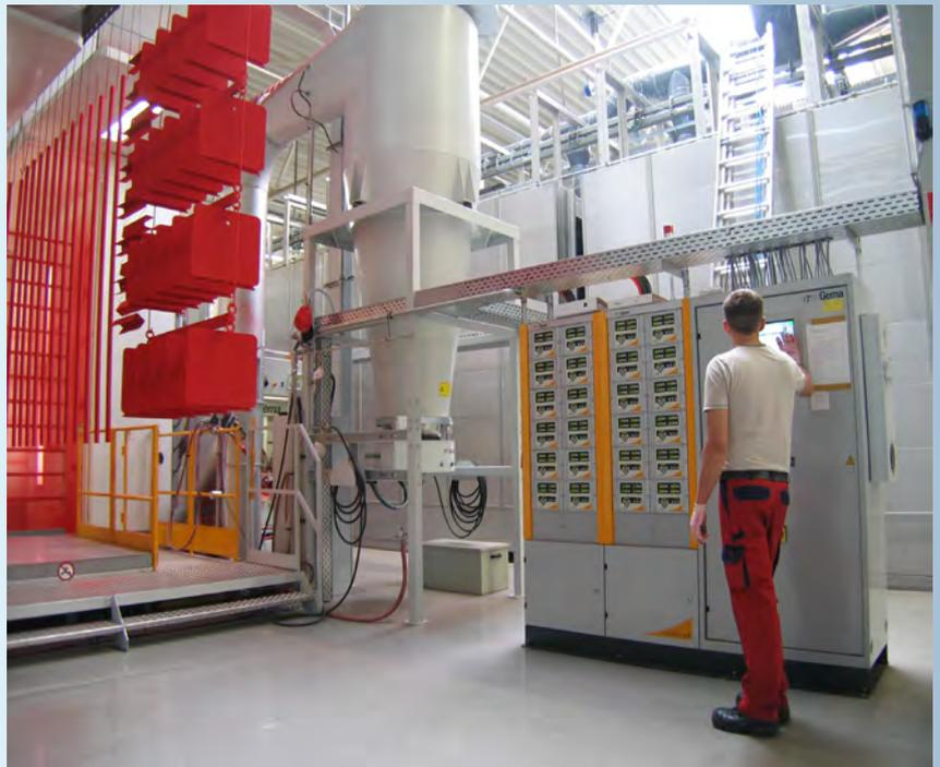
OptiMatic AS02 equipped with 26 control modules OptiStar
