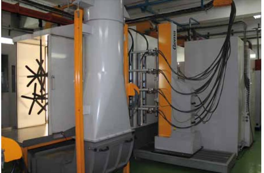
coat as many as 7000 leg assemblies for office chairs in each shift. In addition, two manual coaters can apply a coating to particularly tricky spots either beforehand or afterwards. If more capacity is required, conveyor speed can be increased to 6m/minute and thus an additional 1400 leg assemblies can be coated.
