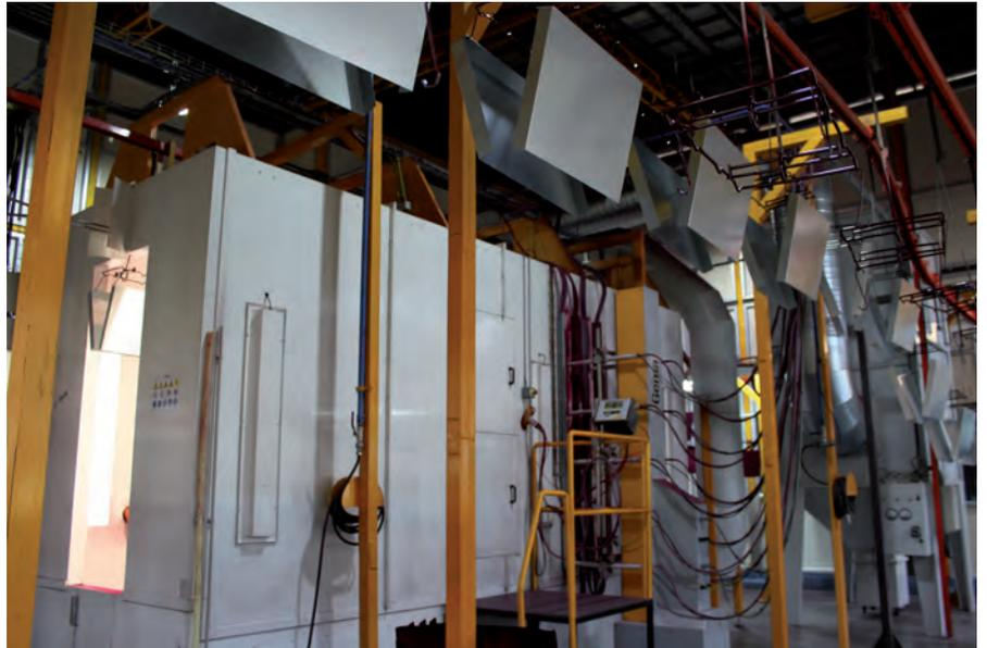
ment. Employees are enthusiastic because they find it much easier to apply the coating as well as to do cleaning compared to the previous coating system. Perfect airflow prevents powder from escaping the system, and the area around the system remains much cleaner.
